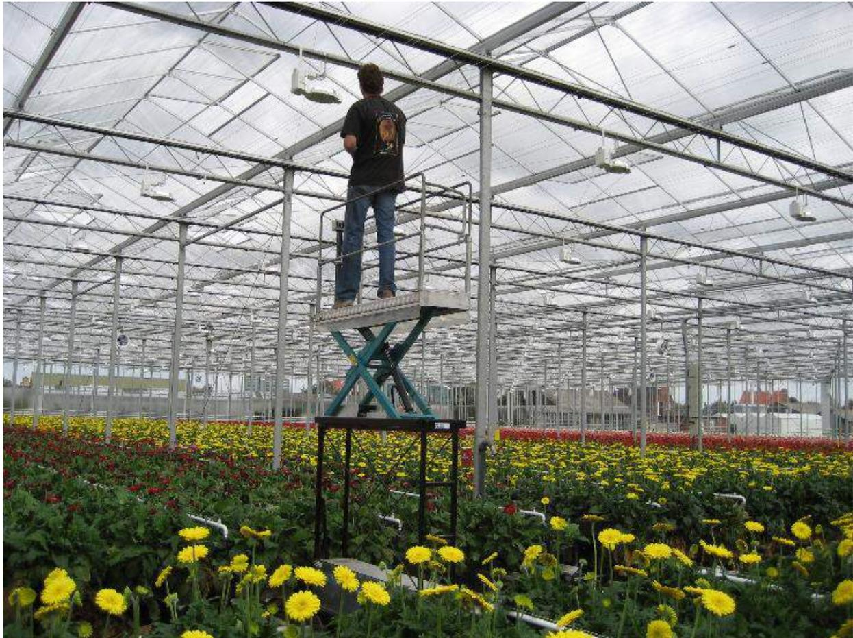
Source : Pipe rail trolley – [www.steenks-service.nl](http://www.steenks-service.nl)
